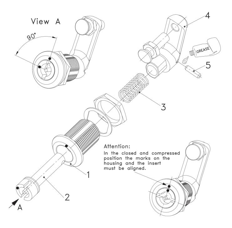
A) Install housing (1) with the mark into direction of the frame.
